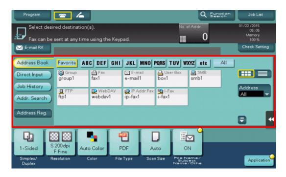
If necessary, you can change the display of the main screen in fax/scan mode (default: [Address Book]). For details, refer to Here.
