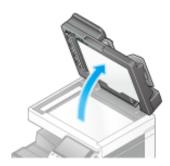
2. Wipe stains off the Slit Scan Glass using a dry and clean cloth.
